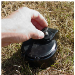
Figure 12 Placing Washer on MIU
