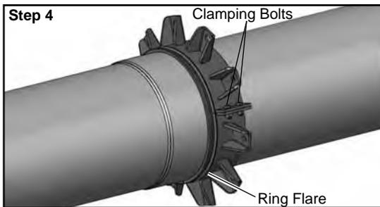
**Step 4.** Loosely assemble (do not tighten the bolts) two ring sections on the spigot side of the pipe with the 1/2" clamping nuts & bolts provided. The flare side of the assembled ring should face the tapered side of the gasket. Assemble the other two ring sections together on the bell side in the same manner.
