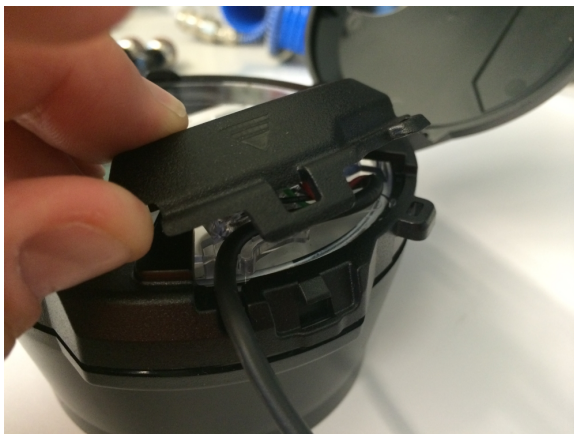
Figure 9 – Covering the Terminal Screws
