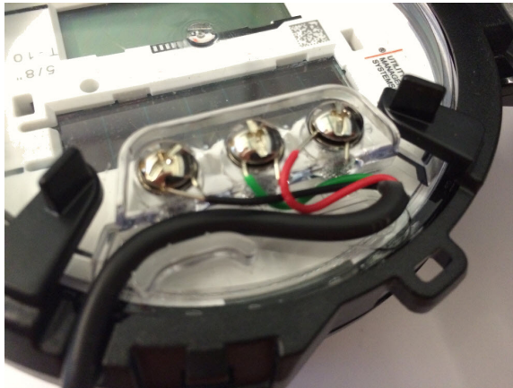
Figure 7 – Cable Threaded Around Strain Relief Posts
