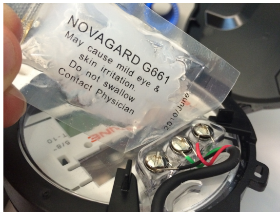
Figure 8 – Application of the Sealant
