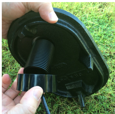
Figure 29 – Locking the Nut on the Antenna
