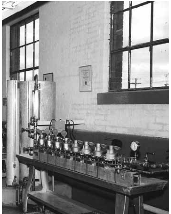
Testing 12 meters in series on an Indianapolis Test Bench. Electric control closes the valves at completion of test.
