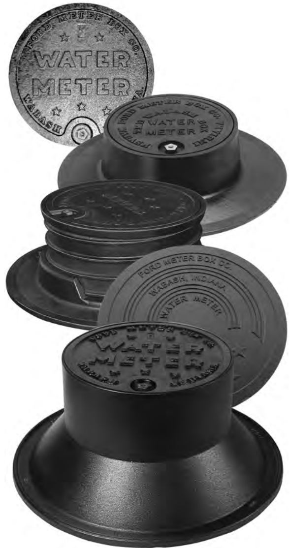
Lids and frames are manufactured from cast iron meeting ASTM A48, Class 25 (25,000 PSI tensile strength).
