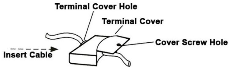
Inserting Multi-Conductor Cable
