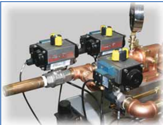
Pneumatically powered inlet valves
