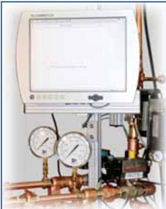
Waterproof touch-screen PC monitor attaches directly to the test bench for easy access
