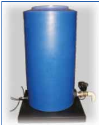
Scale and plastic tank with pneumatically powered drain valve
