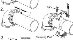
2. Use one of the rods (provided) as a guide, and mark a line on the pipe to position 1300 restrainer. Leave sufficient threads on the rod ends to fully engage nuts. Tighten clamping bolts on each side evenly, to recommended torque (see recommended clamping bolt torque range table), ensuring the gaps between pads on both sides remain even. A torque wrench is required to ensure proper torque. The clamping pads will not touch.
