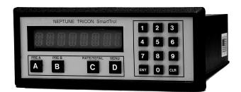
The SmartTrol is a remote instrument designed for flow rate monitoring, totalizing, and batching. It has an 8-digit, 0.55-in bright alphanumeric display. The two inputs (A and B) will accept up to 1,000 pulses per second (pps) of digital count. The two inputs are combined into a single count that can be used to provide a two-stage relay output for valve control.
