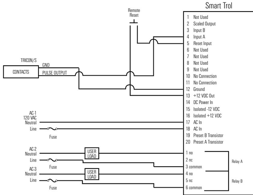
NOTE: The SmartTrol must be ordered from the factory configured for use with the TRICON/S.
