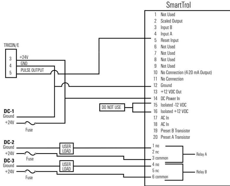
The SmartTrol may be powered by an external DC power supply. The supply must provide 12-27 VDC and at least 250 mA of current. The positive side (+DC) of the supply should be connected to terminal 14 and the negative (or ground) side to terminal 12. Units Powered by DC voltage do not have an isolated voltage on terminals 15 and 16.
