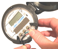
Figure 4: Routing the Wire
