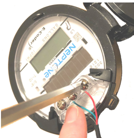
Figure 3: Wiring with Proper Color Wire
