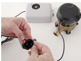
Figure 15: Gray Wires in Slot
