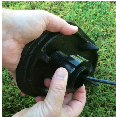
Figure 9 – Securing the Locking Nut
