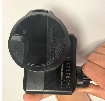
Figure 13 – Connecting the Coaxial Cable
