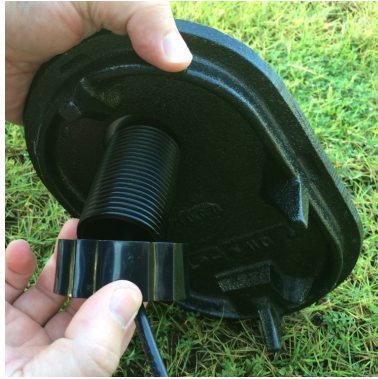
Figure 8 – Locking the Nut on the Antenna
