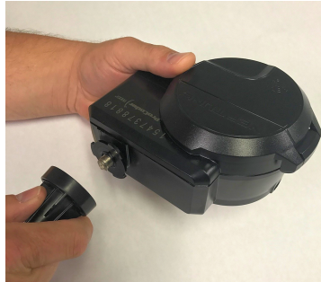
Figure 12 – Aligning the F Connector
