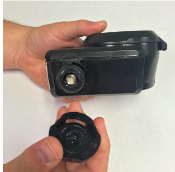
Figure 11 – Removing the Dust Cover
