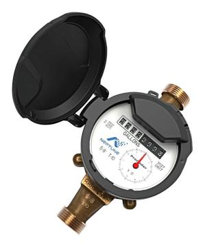
The Neptune® ProCoder<sup>™</sup> solid state absolute encoder register features a high-resolution, mechanical sweep hand to detect ultra-low flows as well as monitor direction of flow. The ProCoder's non-contact LED absolute encoding technology ensures the odometer read exactly matches the remote read. It provides a high-resolution, 8-digit remote meter reading along with leak, tamper, and reverse flow flags when connected to a Neptune R900<sup>®</sup> System endpoint.
