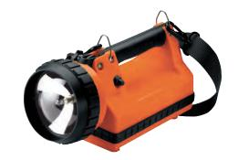
Battery/Run Time: Zero-maintenance 6V, 12Ah sealed lead acid operates up to nine hours per charge and is rechargeable up to 500 times. Red & green LEDs give charge status feedback.
