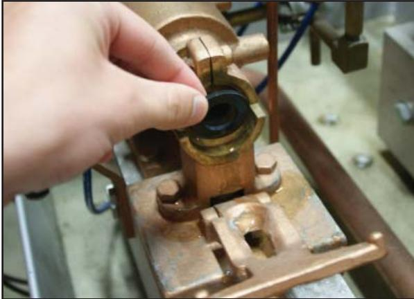
*Install meter adapters and gaskets*
