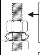
Smith-Blair® Belleville Washers (p/n 150115-000) must be used on PE pipe installations. Use of any other type of Spring Washer may cause product failure.
