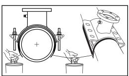
3. Begin tightening the bolts using the pattern shown in the diagram below. Make sure the gap between the sleeve sections is equal on top and bottom and equal from end to end.
