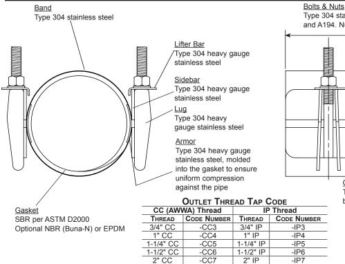
Type 304 stainless steel nuts and washers per ASTM A193 and A194. Nuts are coated to prevent galling.
