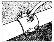
Saddle Installation Slip the saddle around the pipe next to hole and rehook the top and bottom. Make certain the gasket is free of foreign material and there is nothing lodged between the gasket and pipe. Center the saddle over the damaged section. Hand-tighten the nuts evenly. Torque the nuts evenly with incremental torque settings to a maximum of 50-60 ft.lbs. Recheck the saddle bolt torque before back filling.
