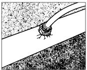
Leak and Pipe Confirmation Confirm the leak location by cleaning and examining pipe. Check the diameter of the pipe to make certain you are using the correct size saddle.
