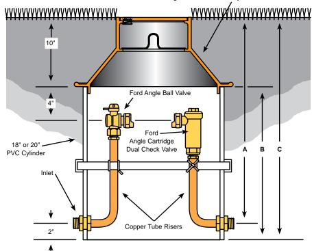
The drawing above shows a Plastic Pit Setter with optional Inlet Angle Ball Valve and Outlet Angle Cartridge Dual Check Valve.
