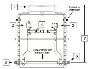
1-1/2" Pit Setter shown with Optional Dual Check Valve in By-Pass
