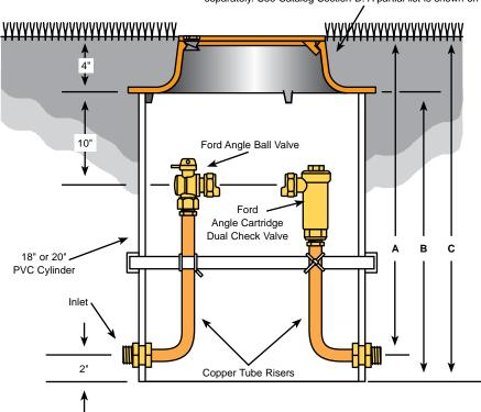
The drawing above shows a Plastic Pit Setter with optional Inlet Angle Ball Valve and Outlet Angle Cartridge Dual Check Valve.
