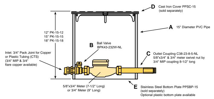
3/4" MALE IRON PIPE INLET BY 3/4" MALE IRON PIPE OUTLET
