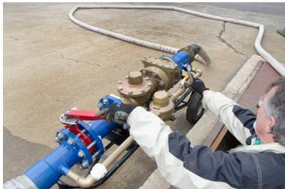
Figure 15 High Side Valve on Reference Meter
