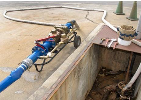
**Figure 6 Connect Fire Hose to Reference Meter**
