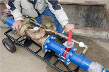
**Figure 7 Purge Air from Test Setup**
