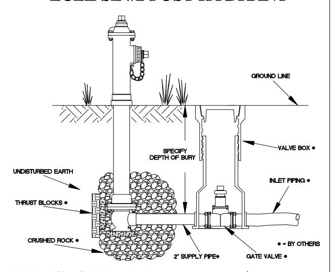
Hydrants shall be self-draining, non-freezing, compression type with 2-1/8" main opening. Inlet shall be (2", 2-1/2" + 3") FNPT, or 2", 3" or 4" MJ). Outlet shall be (3/4") GHT or 1", 1-1/4', 1-1/2', 2' or 2-1/2' MNPT or 1-1/2', 2' or 2-1/2' NST.
