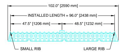
INSTALLED LENGTH ADJUSTMENT = 0.5' (0.15 M) ALL CONTACTOR FIELD DRAIN C-4HD UNITS ARE MARKED WITH A COLORED STRIPE FORMED INTO THE PART ALONG THE LENGTH OF THE CHAMBER.
