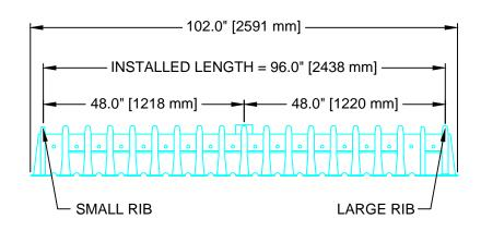
INSTALLED LENGTH ADJUSTMENT = 0.5' (0.15 m) ALL CONTACTOR EZ-24HD UNITS ARE MARKED WITH A COLORED STRIPE FORMED INTO THE PART ALONG THE LENGTH OF THE CHAMBER.
