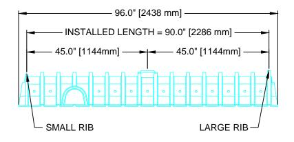
INSTALLED LENGTH ADJUSTMENT = 0.5' [0.15 m] ALL CONTACTOR 100HD HEAVY DUTY UNITS ARE MARKED WITH A COLORED STRIPE FORMED INTO THE PART ALONG THE LENGTH OF THE CHAMBER.
