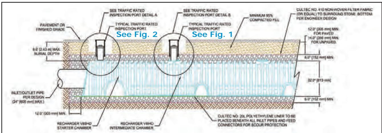
The Recharger V8HD has an 8" (200 mm) diameter inspection port on Model V8SHD Starters, V8RHD Stand Alone and V8EHD End units. The Recharger V8IHD Intermediate unit has a 6" (150 mm) diameter inspection port opening.
