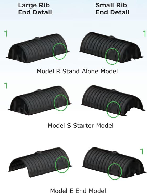
Trimming may only be performed on fully closed endwalls (indicated by Number 1 in Fig. 1) or side portal areas (See green circles in Fig. 1 for side portal locations). Pipe may not be inserted into the sidewall of the chamber unless it is within the side portal trim lines See page 14 for more information on trimming side portals.
