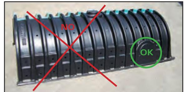
Trimming may only be performed on the side portal area. Side entry in any other location is unacceptable.
