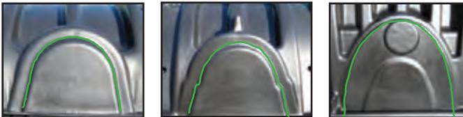
**Shown L-->R:** Guidelines to follow for correct trimming for SFCx2, FC-24 and F-110x4 portals. Do not cut outside of the side portal area guides.
