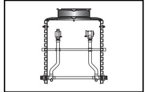
MALE IRON PIPE THREAD INLET AND OUTLET - FOR 2" METER
