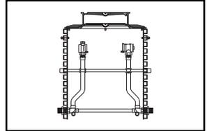
MALE IRON PIPE THREAD INLET AND OUTLET - FOR 1-1/2" METER
