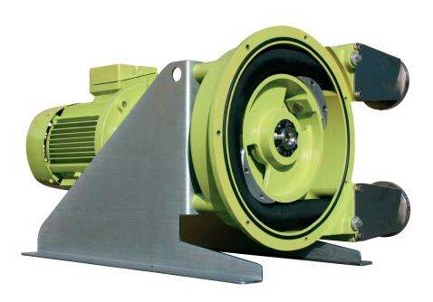
Two shoes mounted at 180° on a rotating wheel successively compress a reinforced rubber hose that contains a fluid to be pumped. The motion of the shoes compress the rubber against the pump housing creating continuous suction at the inlet of the pump and pushing the fluid to the outlet of the pump.
