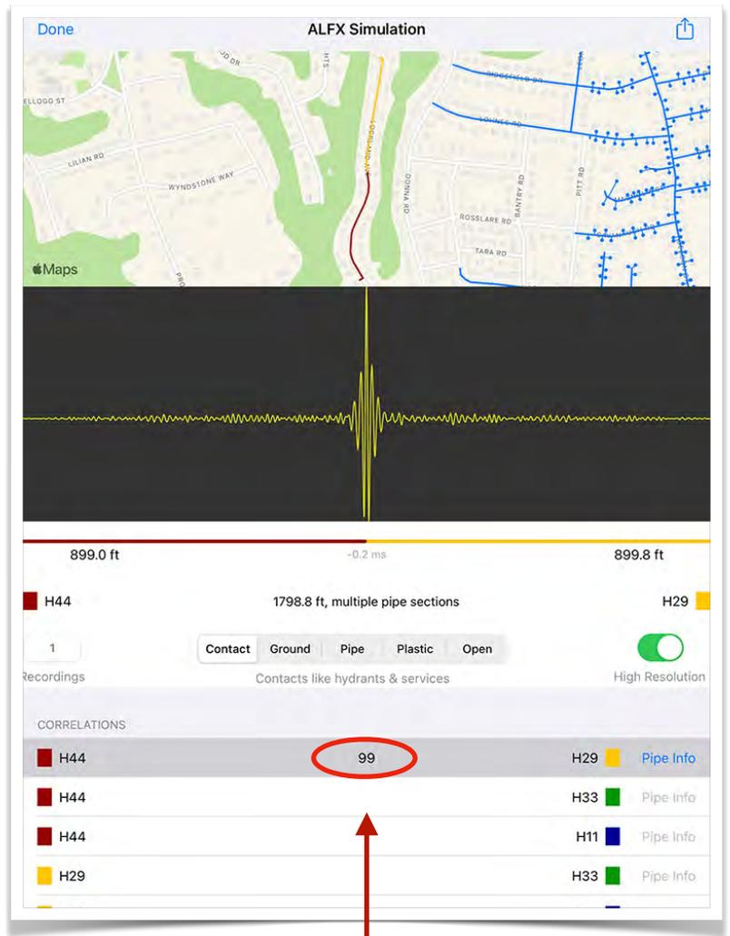
The number in the center of the row is the correlation score which ranges from 0 to 100. The higher the number the higher the confidence in the leak location
