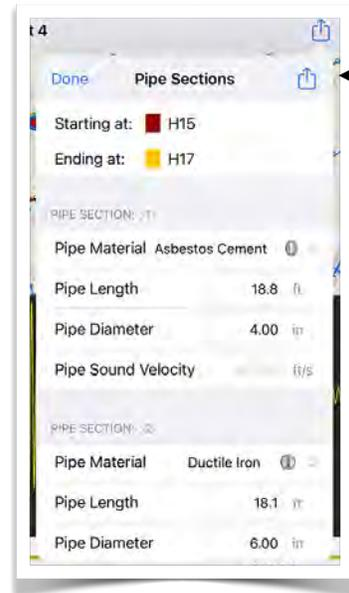
Add another section of pipe by tapping on the Action button and selecting **Add Pipe Section**.
