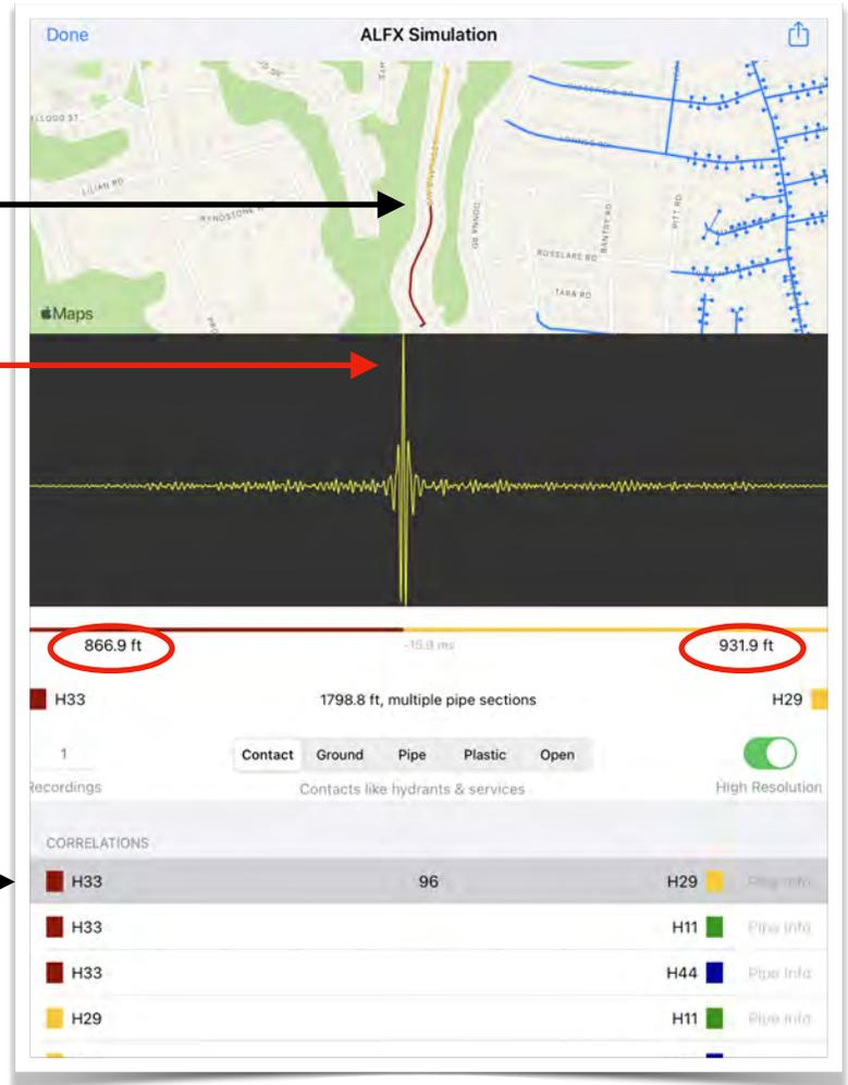
Tap on the Action button in the top right corner to **Set Reference Sensor** and then tap a new reference sensor / hydrant from the list.
