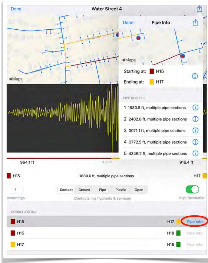
Tap here to view the ALFX sensors installed on these hydrants.
