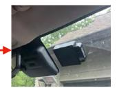
When you have finished surveying or follow-up activities, you can remove the ALFX Controller while leaving the Controller Holder attached to the windshield by sliding the Controller out of the Holder.
