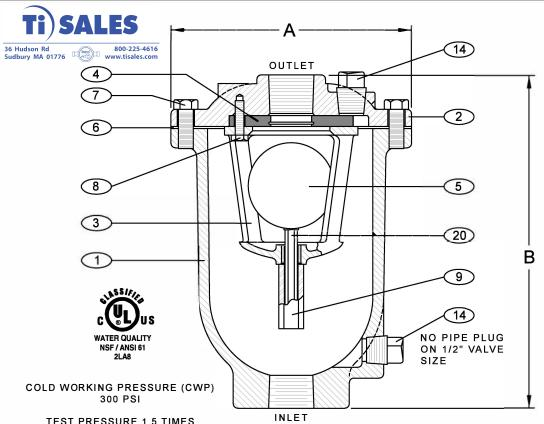
**TEST PRESSURE 1.5 TIMES** COLD WORKING PRESSURE
