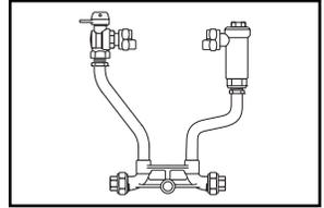
ANGLE BALL VALVE BY ANGLE CARTRIDGE DUAL CHECK VALVE (5/8" METER)
