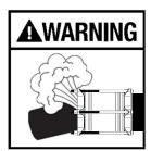
THIS PRODUCT DOES NOT RESTRAIN PIPE MOVEMENT. Proper anchoring is required to prevent pipe pullout. Failure to anchor or improper anchoring can result in dangerous pipe content escape, property damage, serious injury, or death. Read the product installation instructions prior to installing
