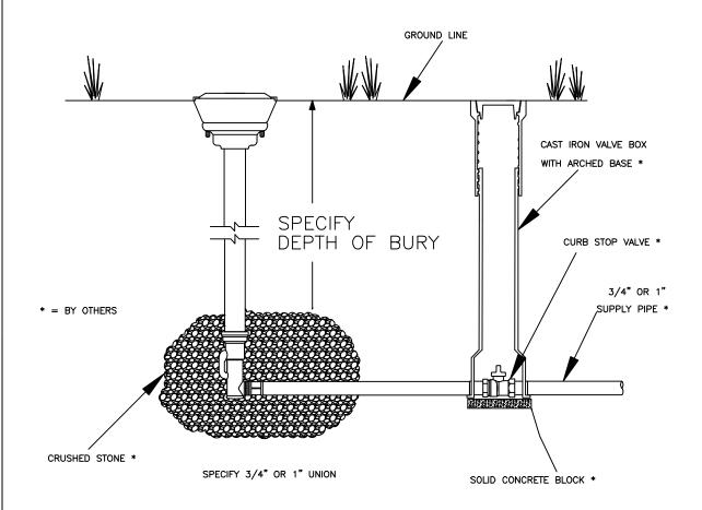
Below grade Ground Hydrants shall be self-draining, non-freezing, compression type. Inlet shall be 3/4" or 1" MNPT. Outlet shall be 3/4" MNPT or GHT, or 1" MNPT.
