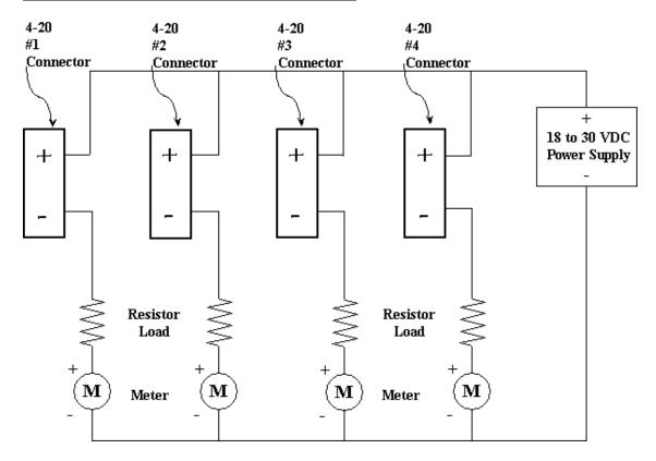
Please note that the power supply in this diagram can range from 18 to 30 VDC. Typical power supplies will be around 24 VDC to this loop powered 4-20 mA circuit. If you have any questions regarding the connections of this unit, please notify the factory.
