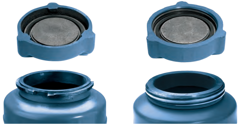
OLD-STYLE CAPS Three lug, 1/3-turn design rated to 200 psi.
